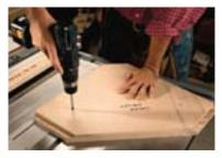
FOr this cherry corner cabinet, I screwed the pattern to the shelf on its sappy underside. A couple brad nails would also do the trick. Align the shortest part of the pattern flush with a jointed or straight-sawn edge.
